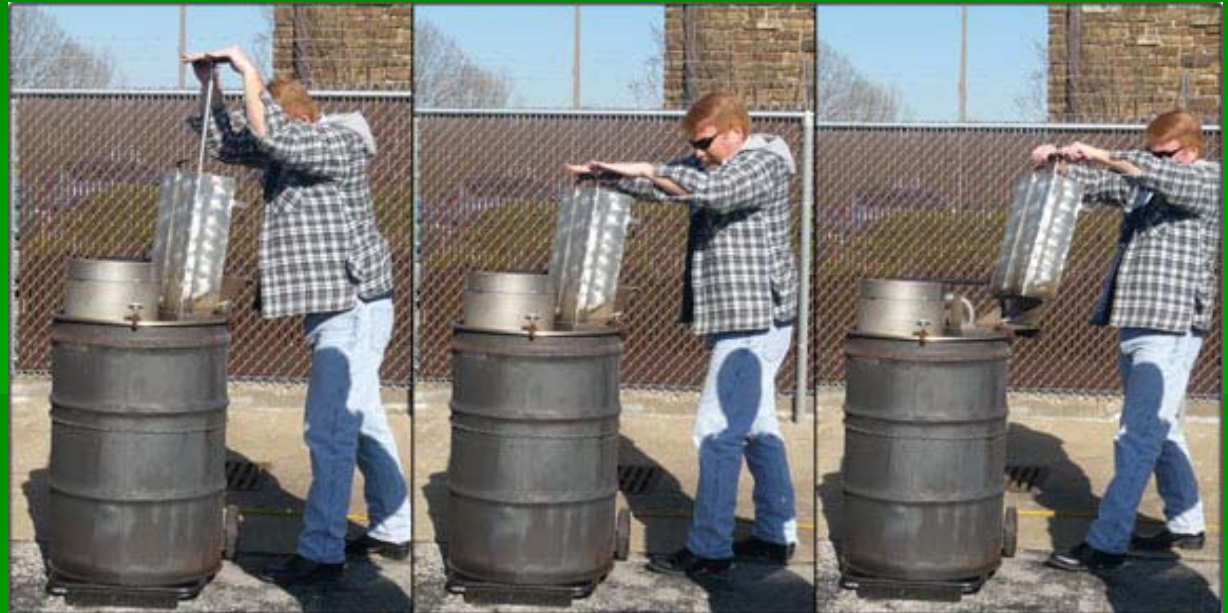
1-2-3... Mark Kruger injects bottles of prescription medication into the Bella Vista, Arkansas, Police Department's Drug Incinerator. The incinerator is used as an alternative to flushing unwanted drugs, which can make their way into the drinking water system.
